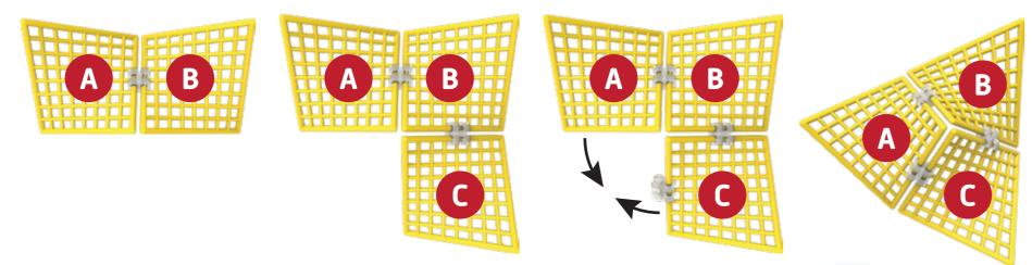
Use a connector to link together tiles A and B.
